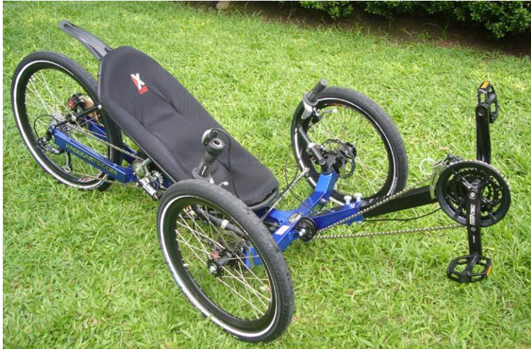
▲ A Cyclone fitted to a recumbent trike using a double-freewheel motor
