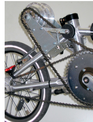
▲ The 'Presto': Cyclone freewheel double-chainwheel powered by a 'nano' hub motor ▼
