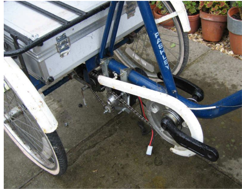
Final fit to the bike with a large battery case for Lead Acid batteries. No eccentric crank is needed because the motor is mounted further back than the Tri-1
