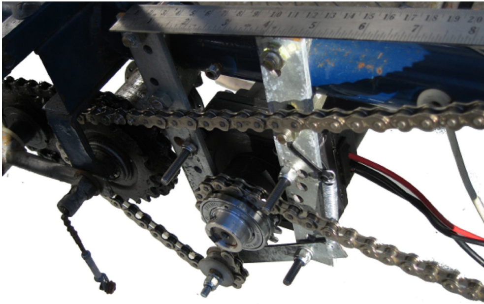
This picture shows the 'first fit' with the motor mounted to the frame with the chain and tensioner.
