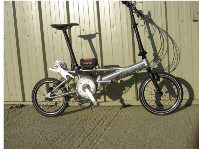
▲ The 'Presto': Cyclone freewheel double-chainwheel powered by a 'nano' hub motor ▼
