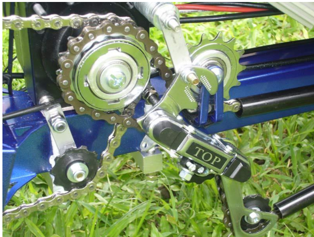
▲ A Cyclone fitted to a recumbent trike using a double-freewheel motor
